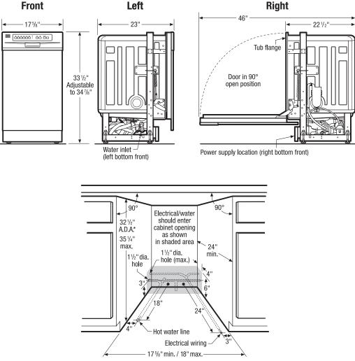
\*A.D.A. installation, (321/2") beneath 34"- high countertop may be accomplished by adjusting toekick and leveling legs.
