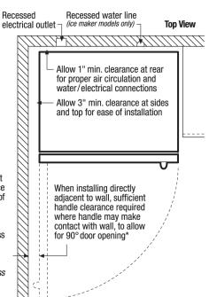
\* When installing freezer adjacent to wall, cabinet or other appliance that extends beyond front edge of unit, 20" minimum clearance recommended to allow for optimum 140° door swing, populatin 140 door swing, providing complete basket access and removal. (Absolute 3" minimum clearance will ONLY allow for 90° door swing which will provide limited basket access with restricted removal.)
