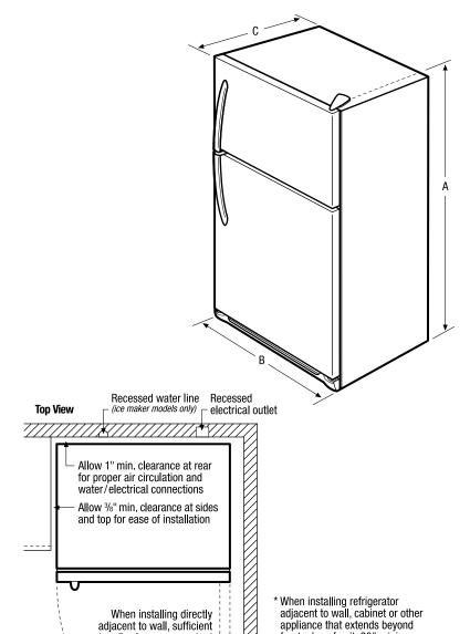
adjacent to wall, cabinet or other appliance that extends beyond front edge of unit, 20" minimum clearance recommended to allow for optimum 140° door swing, providing complete crisper access and removal. (Absolute 3" minimum clearance will ONLY allow for 90° door swing which will provide limited crisper access with restricted removal.)
