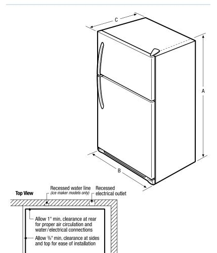
\* When installing refrigerator adjacent to wall, cabinet or other appliance that extends beyond front edge of unit, 20" minimum clearance recommended to allow for optimum 140° door swing, providing complete crisper access and removal. (Absolute 3" minimum clearance will ONLY allow for 90° door swing which will provide limited crisper access with restricted removal.)
