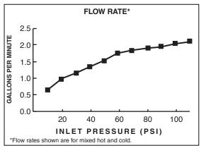
1.8 gpm/6.8 L/min. FLOW RATE
