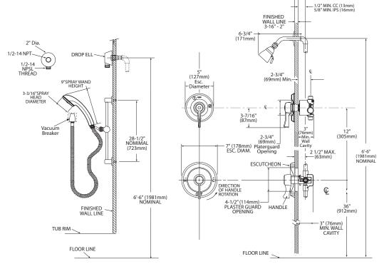
NOTE: This valve is not intended to be used as a shut-off valve. To prevent the potential of cross flow, check valves must be integral to the supply valve or installed in both hot and cold water supply lines.
