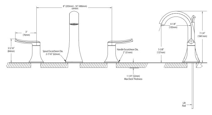
NOTE: FOR DECK THICKNESS 1-3/8" - 3", USE SERVICE KIT #115001. VALVES INSTALL THROUGH 1-1/4" DIA. HOLE
