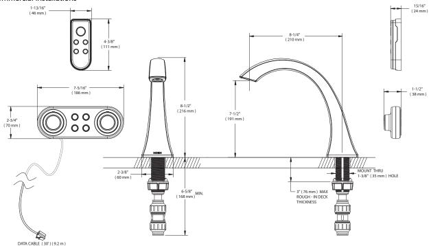
NOTE: THE INSTALLATION SHOWN IS FOR TILE DECKS, THIS VALVE WILL ALSO FIT STEEL, CAST IRON OR PLASTIC DECKS **CRITICAL DIMENSIONS**
