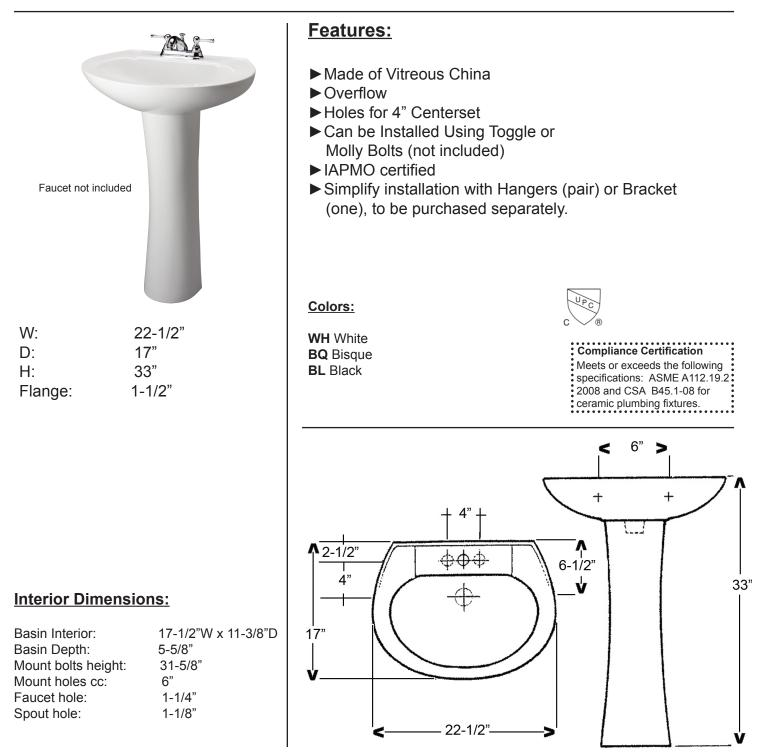
Dimensions of fixture are nominal and may vary within the range of tolerances established by ASME Standard A112.19.2-2008. Dimensions and specifications subject to change without notice.
