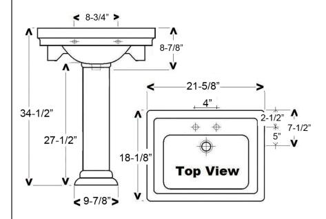
Dimensions of fixture are nominal and may vary within the range of tolerances established by ASME Standard A112.19.2-2008. Dimensions and specifications subject to change without notice.
