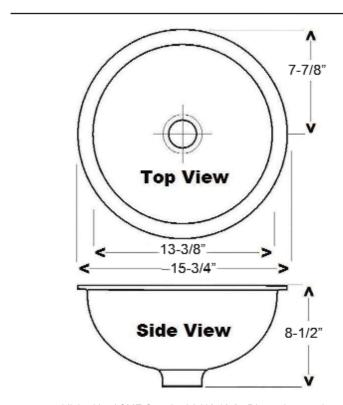
Dimensions of fixture are nominal and may vary within the range of tolerances established by ASME Standard A112.19.2. Dimensions and specifications subject to change without notice.
