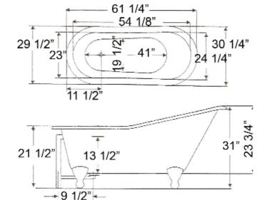
Dimensions of fixture are nominal and may vary within the range of tolerances established by ANSI Standard A112.19.1M. Dimensions and specifications subject to change without notice.
