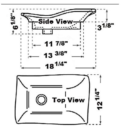
Dimensions of fixture are nominal and may vary within the range of tolerances established by ANSI Standard A112.19.2-2008. Dimensions and specifications subject to change without notice.
