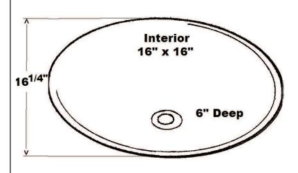
Dimensions of fixture are nominal and may vary within the range of tolerances established by ANSI Standard A112.19.2-2008. Dimensions and specifications subject to change without notice.
