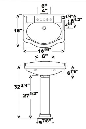
Dimensions of fixture are nominal and may vary within the range of tolerances established by ASME Standard A112.19.2-2008. Dimensions and specifications subject to change without notice.
