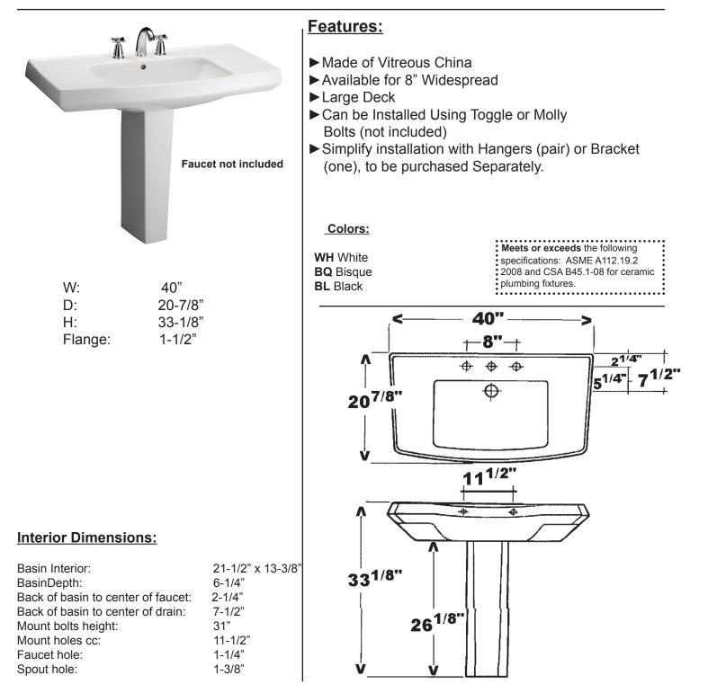
Dimensions of fixture are nominal and may vary within the range of tolerances established by ASMEI Standard A112.19.2-2008. Dimensions and specifications subject to change without notice.
