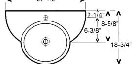
Dimensions of fixture are nominal and may vary within the range of tolerances established by ASME Standard A112.19.2-2008. Dimensions and specifications subject to change without notice.
