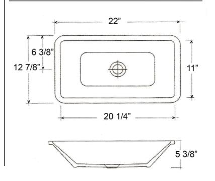
Dimensions of fixture are nominal and may vary within the range of tolerances established by ASME Standard A112.19.2. Dimensions and specifications subject to change without notice.
