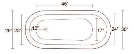
Dimensions of fixture are nominal and may vary within the range of tolerances established by ANSI Standard A112.19.1M. Dimensions and specifications subject to change without notice.
