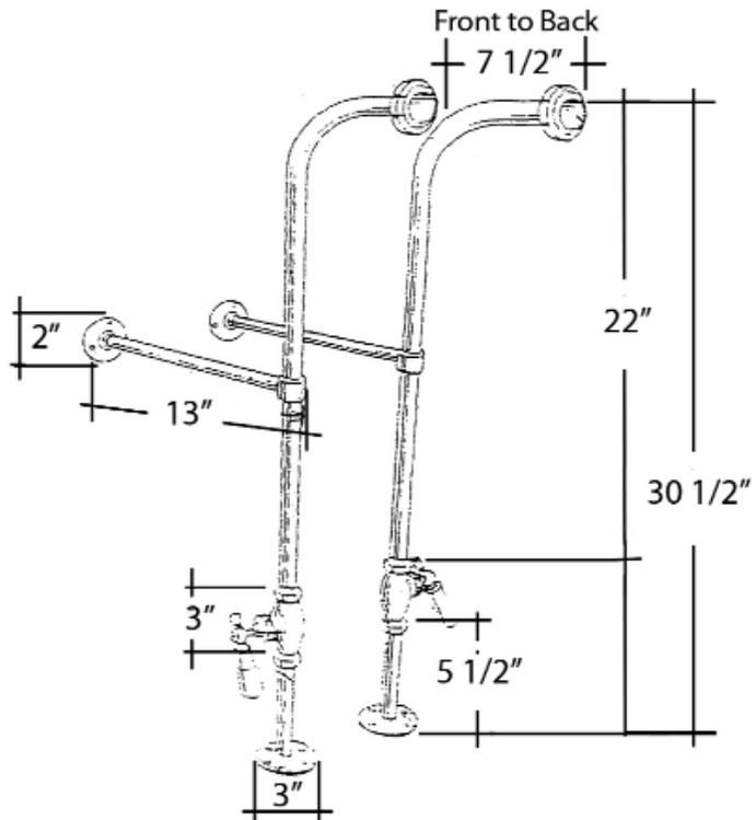
**Use on concrete floors requires special installation. We recommend using a plumbing professional.**
