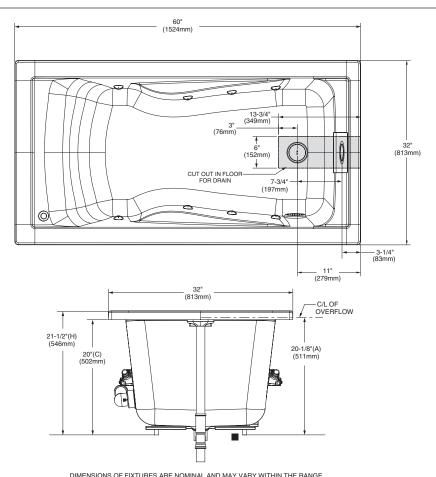
DIMENSIONS OF FIXTURES ARE NOMINAL AND MAY VARY WITHIN THE RANGE OF TOLERANCES ESTABLISHED BY ANSI STANDARDS Z124.1 AND A112.19.7.
