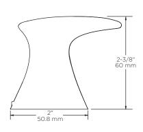
MATERIALS: Base Plate, Post - Zinc Die Cast Wall Plate - Steel, Zinc Plated
