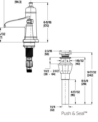
Ø1-1/4 Min to Ø1-1/2 Max. Deck Hole Openings
