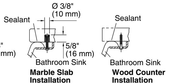
**Note:** Waterproof unprotected overhang area on the underside of wood counter.
