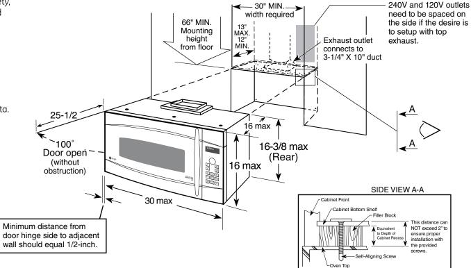
Note: Outside venting is optional. Vent (duct) can be horizontal or vertical.
