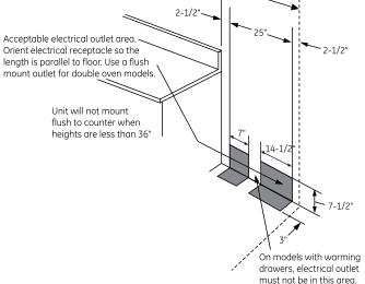
**NOTE:** Use a 4' power cord to prevent interference with unit when installing.
