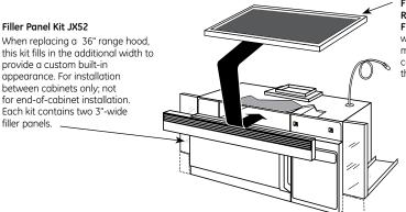
Filter Kit JX81H– Recirculating Charcoal Filter Kit To be used when the Spacemaker microwave oven cannot be vented to the outside.
