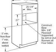
• Oven overlaps will conceal cut edges on all sides of the opening. **Note:** PSB9120 series Advantium can be installed below GE/GE Profile non-downdraft gas and electric cooktops. It CANNOT be installed below induction or Monogram (2GU3841385) gas cooktops.
