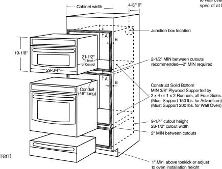
**Note:** Advantium wallovens can be installed below GE/GE Profile Series nondowndraft gas and electric cooktops. It CANNOT be installed below induction or Monogram (2GU3841385) gas cooktops.
