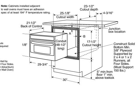
A= Allow 1" overlap of oven over bottom edge of cutout, and allow 1-1/4" overlap at top edge of cutout.
