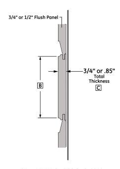
SIDE VIEW CROSS SECTION (Showing Raised Panel with Middle Rail)
