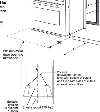
ATTENTION INSTALLER: All electric wall ovens must be hard-wired (direct-wired) into an approved junction box. A plug and receptacle is NOT permitted on these products.
