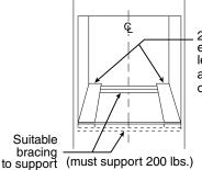
2 x 4 or equivalent runners level with bottom of cutout and flush with sides of cutout or solid bottom floor.
