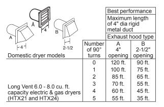
For every extra 90° elbow, reduce the allowable vent system length by 10 ft. Two 45° elbows will be treated like one 90° elbow. For the side exhaust installations, add one 90° elbow to the chart. When calculating the total vent system length, you must add all the straight portions and elbows of the system (including the transition duct). Laundry Center length includes factory-installed elbow that does not impact vent length.
