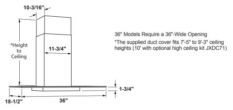
The vent hood must be installed 24" min. above the cooking surface. For optimal performance, installing the hood more than 36" above the cooking surface is not recommended. The hood installation height above the cooking surface depends upon ceiling height. The telescopic duct cover conceals the ductwork running from the top of the hood to the ceiling.
