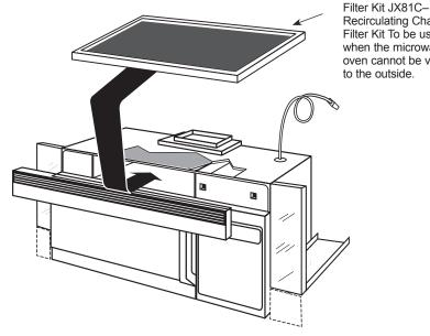
Recirculating Charcoal Filter Kit To be used when the microwave oven cannot be vented to the outside.
