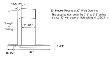
The vent hood must be installed 24" min. above the cooking surface. For optimal performance, installing the hood more than 36" above the cooking surface is not recommended. The hood installation height above the cooking surface depends upon ceiling height. The telescopic duct cover conceals the ductwork running from the top of the hood to the ceiling.
