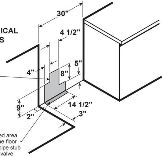
Recommended area for through-the-floor connection of pipe stub and shut-off valve.
