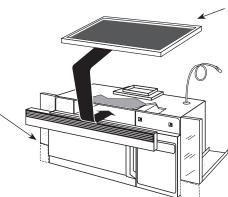
Filter Kit WB06X10807 Recirculating Charcoal Filter Kit To be used when the microwave oven cannot be vented to the outside.
