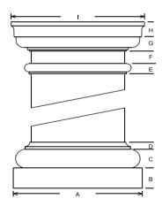
Cap and base sets include neck moulding (customer installed) and installation hardware. These cap & base sets are not for use with other Poly-Classic columns due to shaft size differences. The pultruded mouldings are factory mitered, and assembled into one unit for easy installation. TimeSaver 8" sets are one-piece ABS or polystyrene.
