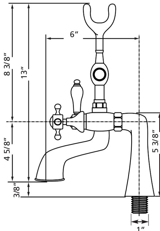
\* Pay close attention to the offset mounting legs. Although the faucet is a 6" spread, the mounting legs install into a 7" spread.
