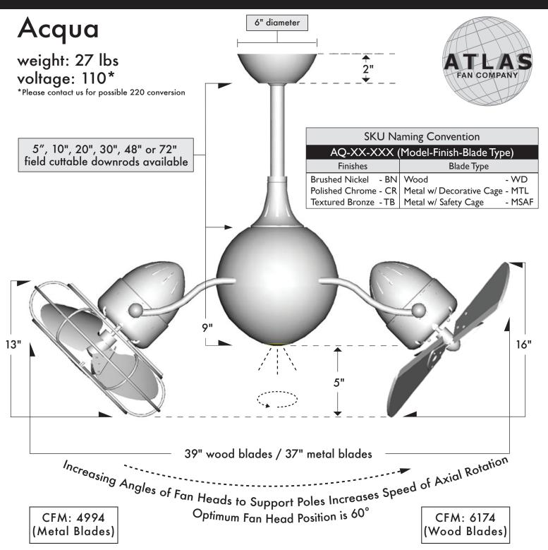
The Acqua can be mounted with any one of the following downrod lengths: 5, 10, 20, 30, 48 or 72".
