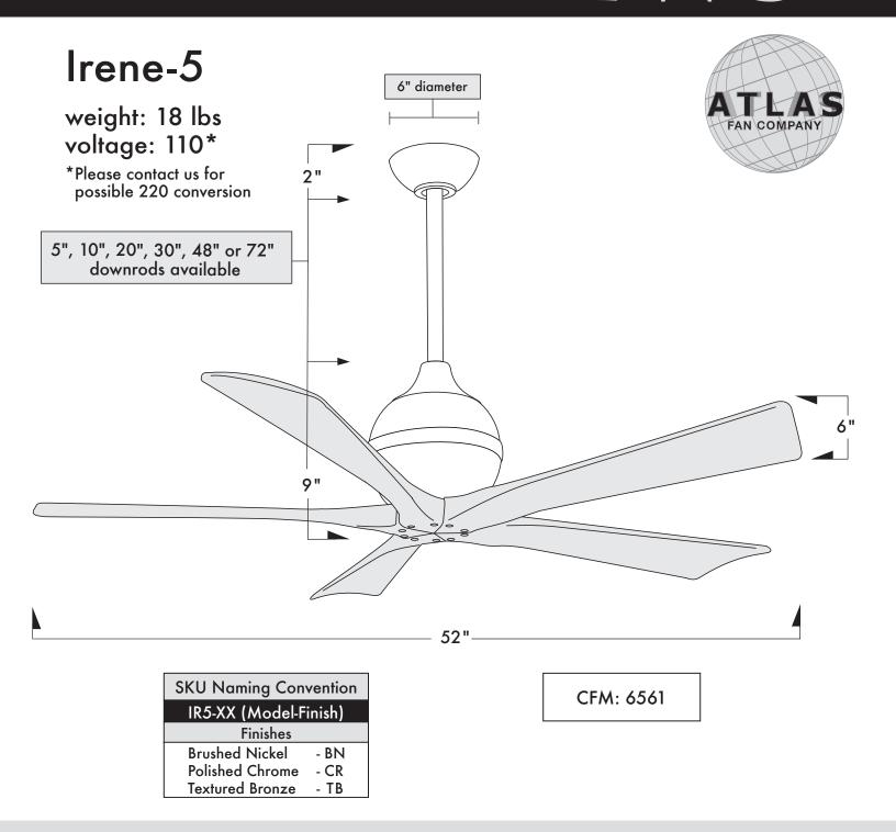
The Irene-5 is compatible with flat or vaulted ceilings and can be mounted with any one of the following downrod lengths: 5", 10", 20", 30", 48" and 72".
