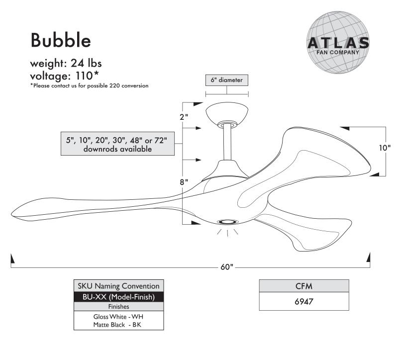
The Bubble is compatible with flat or vaulted ceilings and can be mounted with any one of the following downrod lengths: 5", 10", 20", 30", 48" and 72".
