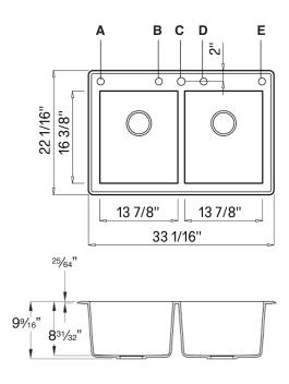
IMPORTANT: Circle Letter(s) above to indicate location(s) for faucet hole drillings (there is a 4" spread between hole locations B,C,D. There is a 10<sup>25</sup>/<sub>64</sub>" spread between hole locations A and B and D and E).
