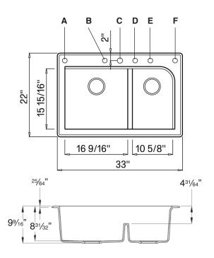
IMPORTANT: Circle Letter(s) above to indicate location(s) for faucet hole drillings (there is a 4" spread between hole locations B,C,D,E. There is a 1033/64" spread between hole locations A and B and 617/32" between E and F).
