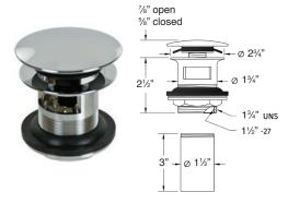
EZ-click™ drain with overflow. Includes 1-1/2" x 3" tailpiece. Fits 2" diameter drain opening. For use with FUSB242010 Quinn Belfast Sink with weir overflow. Lifetime warranty on clicking mechanism.
