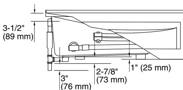
No change in measurements with drain shown. (K-7161-AF or K-7161M-AF)
