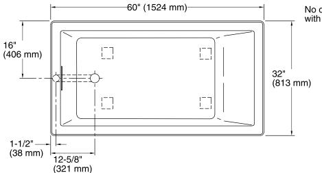
No change in measurements if connected with drain illustrated. (K-7272)
