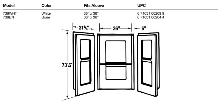
**General:** Furnish and install as shown on plans, 36" square shower, DURAWALL<sup>®</sup> Shower Walls Model 736, as manufactured by E.L. Mustee & Sons, Inc. Shall be 3-piece, molded fiberglass wall with minimum thickness of 125 mils and mounts direct-to-studwalls. Includes center panel with molded-in shelves and two side panels with molded-in shelf. Self aligning panels use a tongue-and-groove connection. Shall meet ANSI Z 124-2011.2. Color\_\_\_\_\_ (White, Bone).
