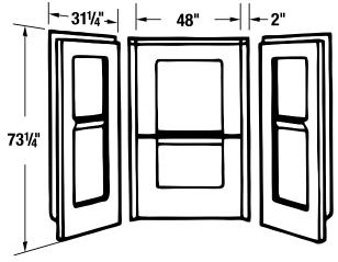
General: Furnish and install as shown on plans, 32" x 48" rectangular shower, DURAWALL® Shower Walls Model 748-32, as manufactured by E.L. Mustee & Sons, Inc. Shall be 3-piece, molded fiberglass wall with minimum thickness of 125 mils and mounts direct-to-studwalls. Includes center panel with molded-in shelves and two side panels with molded-in shelf. Self aligning panels use a tongue-and-groove connection. Shall meet ANSI Z 124-2011.2. Color\_\_\_\_(White, Bone).
