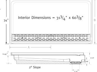
Trough system drains into standard 2" drain pipe.
